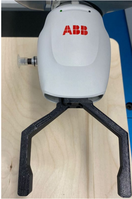
Figure 4.7 New Fingers for cup-grabbing.
