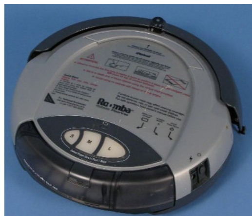
Figure 2.11 Roomba- Automatic Robot Vacuum Cleaner (The National Museum of American History, n.d.)
