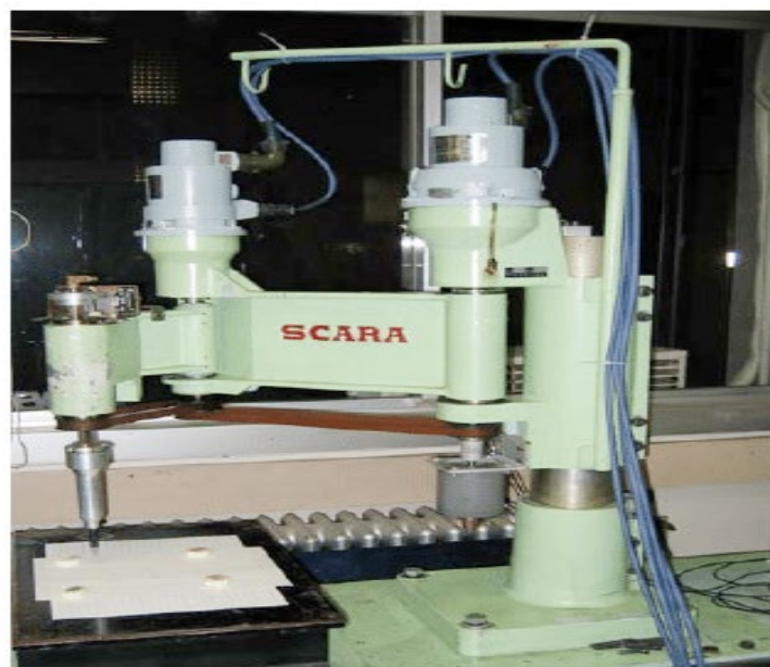
Figure 2.7 The initial SCARA robot prototype (Gasparetto & Scalera, 2019b).
