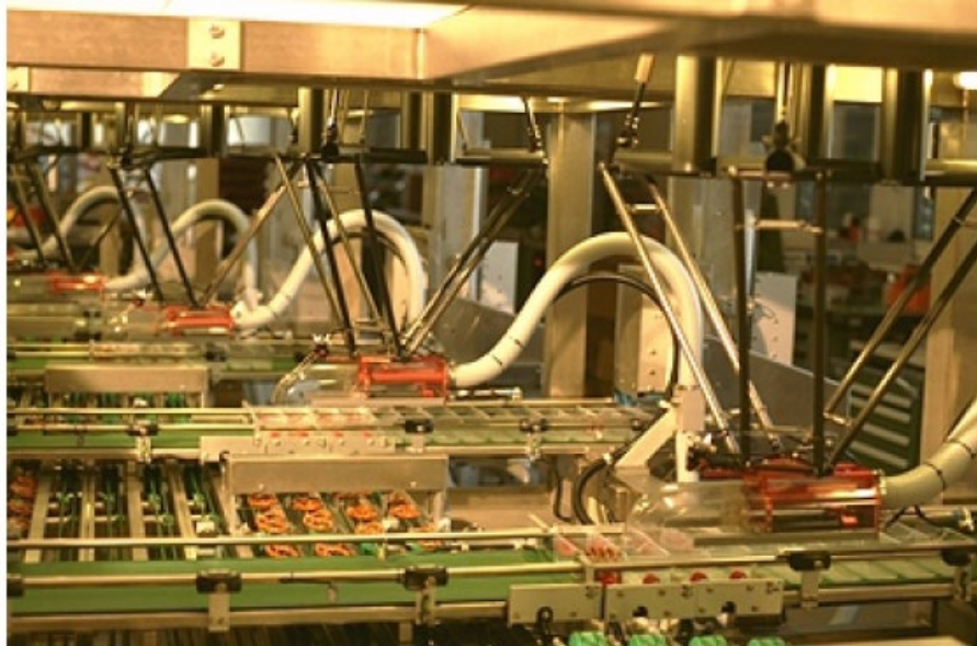
Figure 2.9 Delta robots automate pretzel packaging at Demarex work cells. (Gasparetto & Scalera, 2019a)
