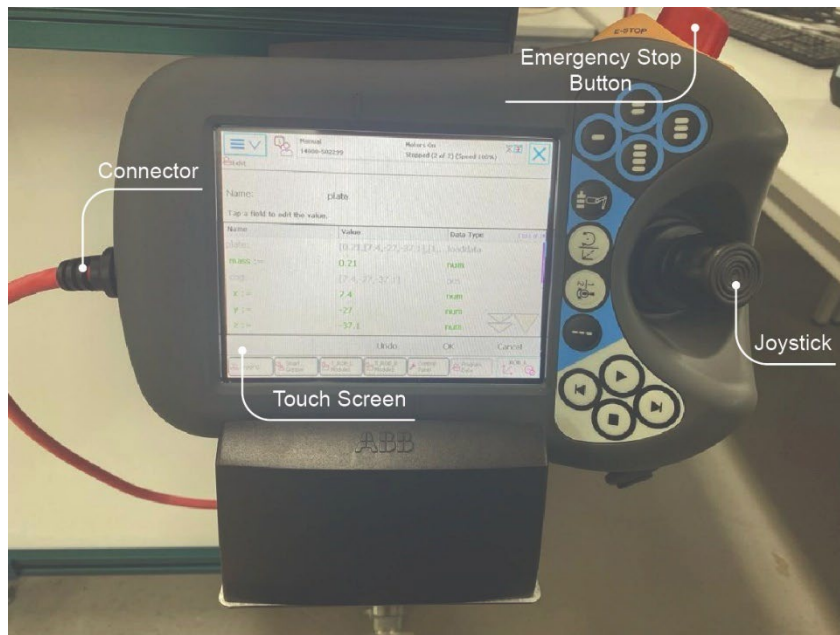
Figure 4.3 Main parts of FlexPendant
